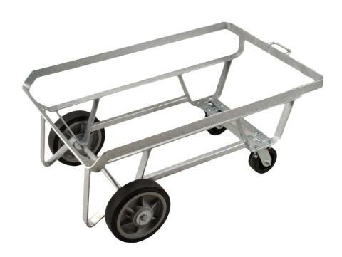
This tall, galvanized steel undercarriage features caster wheels that are impervious to meat fat and bearings equipped with grease fittings. This model includes a built-in stop that allows the tub to be tipped and emptied. This tub accessory is commonly used for meat, seafood, poultry, commercial fishing, confectionery, bakery, and grain applications. Replacement casters and wheels are available.
